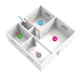
The "foul" air is extracted from the so-called "technical" premises of the house (bathroom, kitchen...) and through suitable ducts connected to the plenum reaches the TEMPERO ECO IL E BP PPE recovery unit where the heat exchange occurs by mixing with the fresh air before being exhausted.
